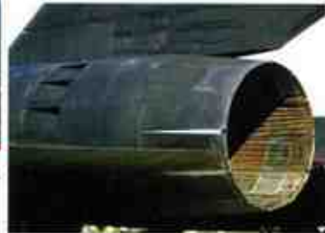
Above: The Blackbird's office was off limits for photography for many years. This photo was taken just before the Blackbird stood down and was legal at the time. (Photo by Ted Carlson/Fotodynamics.com) Right: The afterburning J58 engine was unique to the Blackbird and it even used a very high-temperature oil that solidified at ambient temperatures. Electric heaters were used to liquefy the oil before engine start. (Photo by Ted Carlson/Fotodynamics.com)
